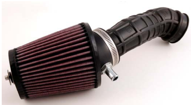
Intake pipe attached to filter.
